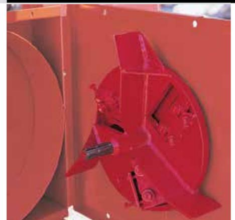
The new modern design of tractor mounted HJ-170 chipper includes separate frame and several user friendly details. Chipper is available as M-model with no separate feeding device and also as G-model which is seen in the picture. The safety of user is secured also in the M-model with a patented feed stopper operated with the control handle.
