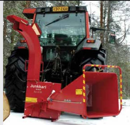
↑ The HJ-4 M model is a mechanical chipper with no separate feeding device. It is particularly well-suited for chipping branchless trees and trees with only a few branches.
