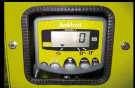
No Stress control Wizard C. The rotational guard of the manual feed chipper also features other practical functions such as an hour counter and a maintenance alarm.
