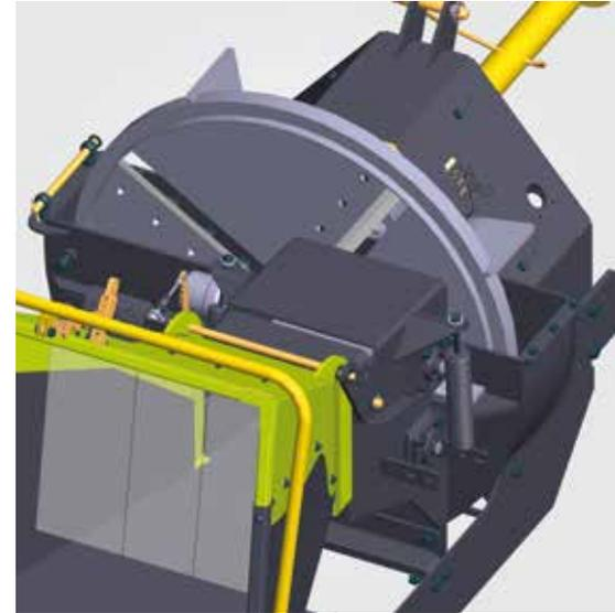
The discs of the HJ-250 and HJ-261 model come with four blades you can adjust continuously depending on the desired woodchip size. The blow wings will finalise the woodchips and blow the chips effectively to the desired location through an adjustable discharge chute.
