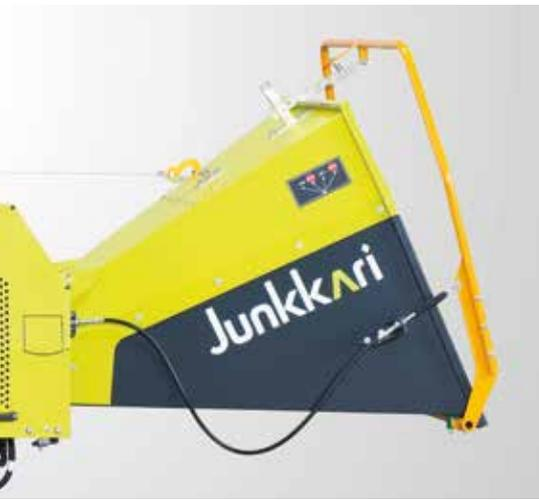
↑ The HJ-250 G model is a chipper with a hydraulic feeding device. Its two feed rollers are powered by the tractor's hydraulics. The HJ-250 GT model is almost identical to it: the only difference is that its feeding device has an independent hydraulic tank and pump. This means that no additional hydraulics is needed.
