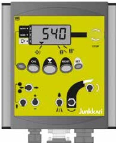
↑ All of Junkkari's chippers that provide loader feeding come with a new Wizard C+ control unit as standard. This unit is used to control the direction of the discharge chute, the feed rollers and the No-Stress rotation guard. The feed rollers can also be controlled with foot pedals.
