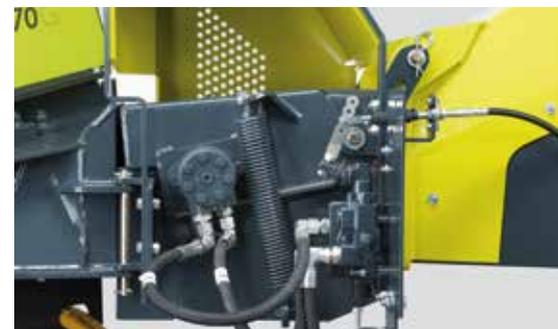
↑ In the picture you can see a hydraulic feeding device of HJ-170 G. It has one feed roller powered by the tractor's hydraulics. The handle is used to control the rotation of the feed roller.
