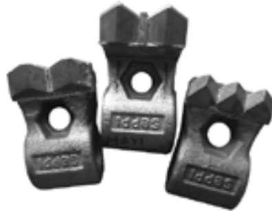
fixed knives with different types of tungsten carbide tips
