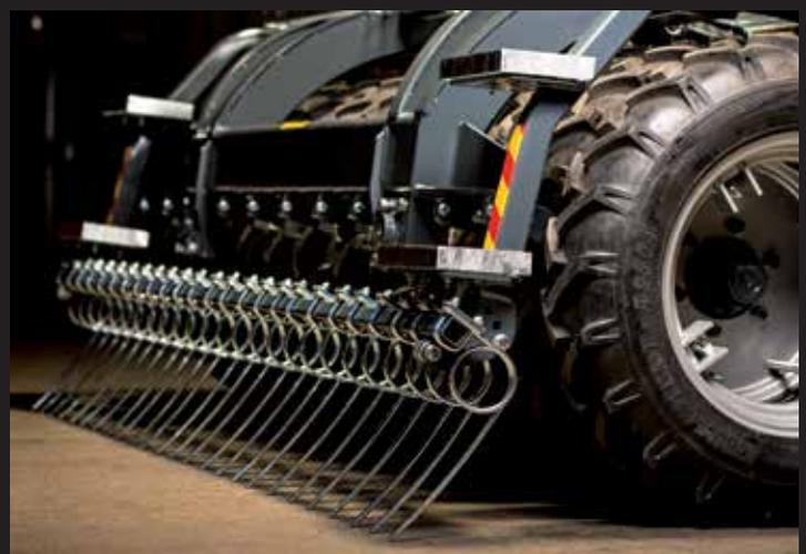
All models can be equipped according to customer needs with either 7,5x16 inch or 7,5x20 inch tractor pattern wheels. The bigger version is also available with brakes. Following harrow is standard in all models.
